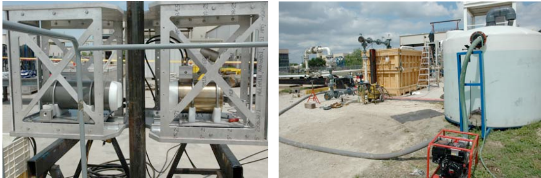
Figure 6. On left, maritized ROV-conveyed Neftemer meter in delivery frame. Flow test setup at SwRI shown on right, with wooden tank for submersion of meter during tests.
