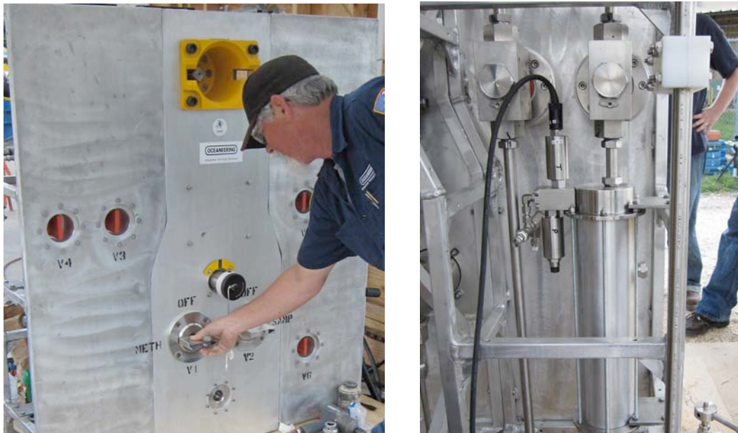
Figure 4. Front and rear of ROV-conveyed sampling panel, sample bottle shown on right.
