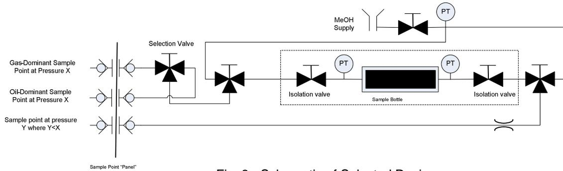
Fig. 3 - Schematic of Selected Design
