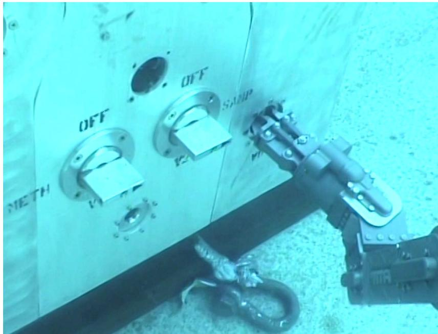
Fig. 12 - Manipulating the Sample System Valves
