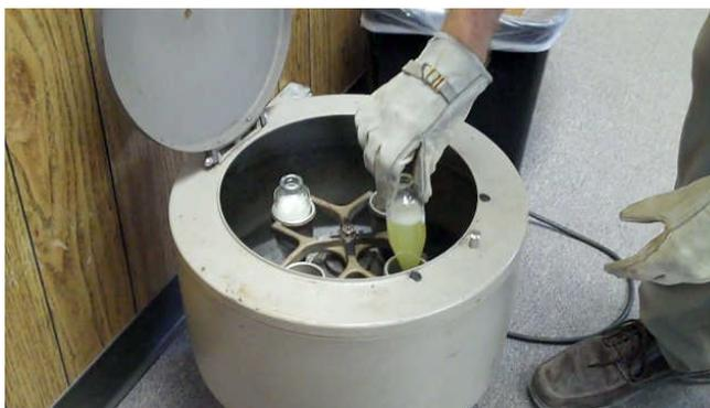
Fig. 7 - Determining Watercut
