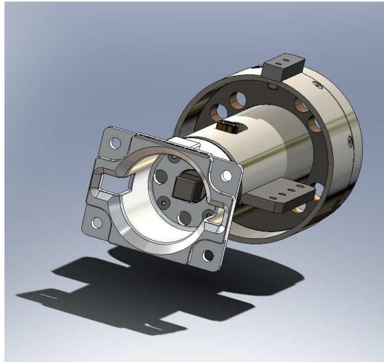
Fig. 5 - Proposed Standard Interface (Coupled)
