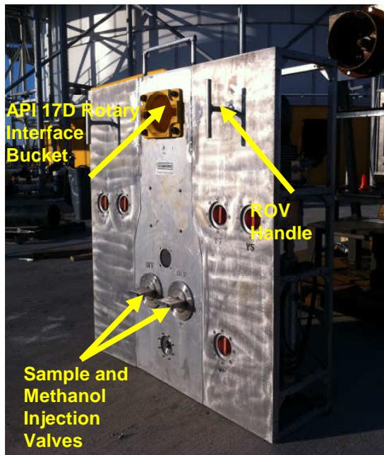
Fig. 4 - Prototype Subsea Sampling System
